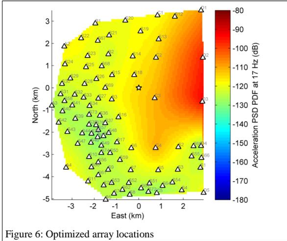
Figure 6: Optimized array locations
