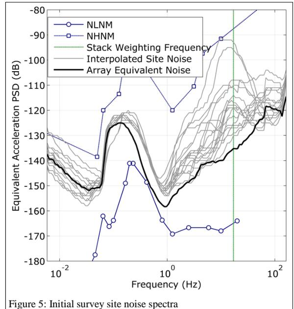
Figure 5: Initial survey site noise spectra
