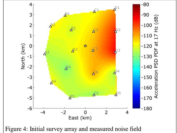
Figure 4: Initial survey array and measured noise field
