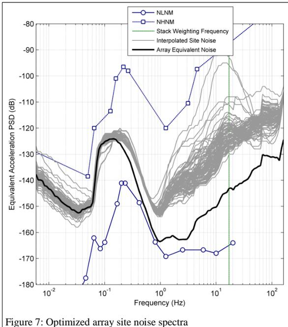
Figure 7: Optimized array site noise spectra
